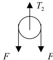
$$\sum F_{//} : 2F - T_2 = m_{polea} \cdot a_{polea} = 0 \Rightarrow T_2 = 2F. \quad (4)$$
