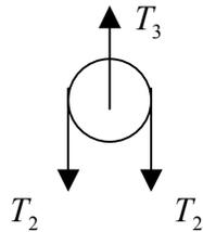
$$\sum F_{//} : T_3 - 2T_2 = m_{polea} \cdot a_{polea} = 0 \Rightarrow T_3 = 2T_2. \quad (3)$$
