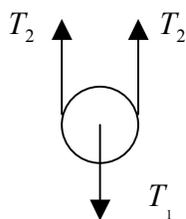
$$\sum F_{//} : 2T_2 - T_1 = m_{polea} \cdot a_{polea} = 0 \Rightarrow T_1 = 2T_2 \quad (2)$$
